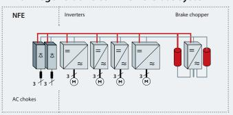
A common DC bus system consists of one or more front-end modules and inverter modules connected together by a DC bus.
