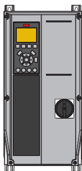
A4 IP55 with mains disconnect
